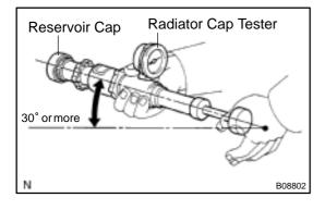
(a) Using a radiator cap tester, slowly pump the tester and check that air is coming from the vacuum valve.
